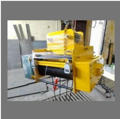
Electric Crane Hoist Capacity 5 Ton
