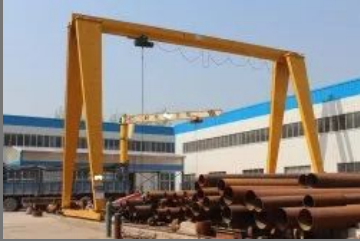
10 Ton Electric Gantry Crane
