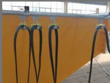
EOT Crane Cable Trolley
